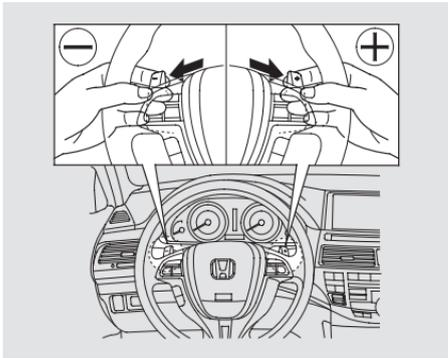
To shift up or down, use the + (right) or - (left) paddle shifter on either side of the steering wheel.
