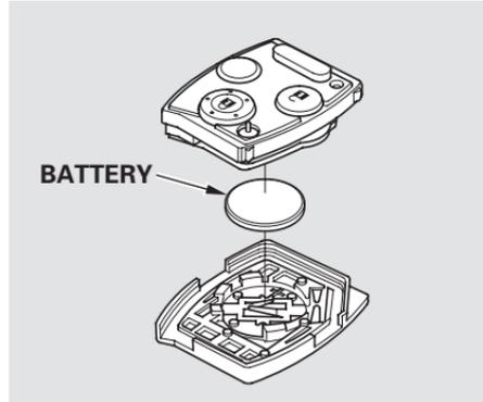
4. Remove the old battery, and insert a new battery into the back of the cover with the + side facing down.
