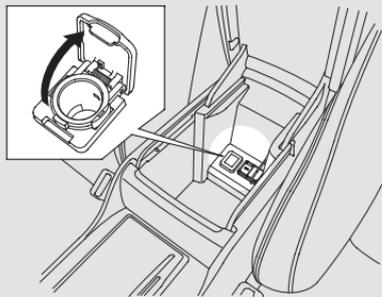
Each socket is intended to supply power for 12 volt DC accessories that are rated 120 watts or less (10 amps).
