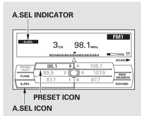
Push the interface selector down to scroll down the screen, highlight A.SEL, then press ENTER on the interface selector. You will see A.SEL on the screen, and the system goes into scan mode for several seconds.
