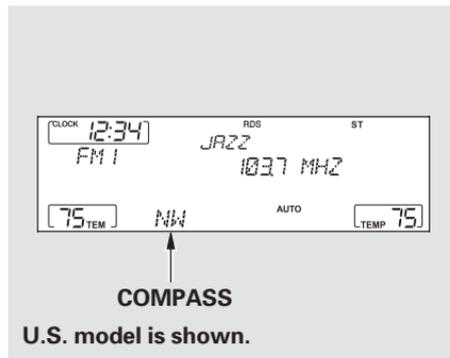
The compass may need to be manually calibrated after exposure to a strong magnetic field. If the compass seems to be continually showing the wrong direction and is not self-calibrating, or the compass display is blinking with the CAL indicator on, do the following procedure.
