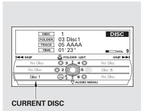
Select the changer by pressing the CD button. The system will begin playing the last selected disc in the disc changer. You will see the current disc position highlighted.
