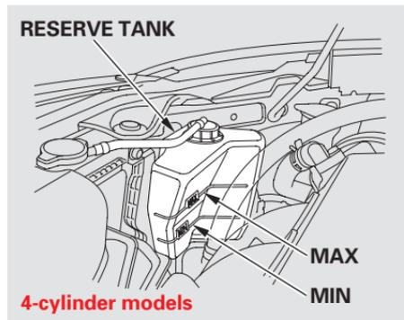
Look at the coolant level in the radiator reserve tank. Make sure it is between the MAX and MIN lines. If it is below the MIN line, see **Adding Engine Coolant** on page 354 for information on adding the proper coolant.
