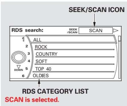
To activate RDS program scan with the interface dial, push the AUDIO button to display the FM radio information on the screen. Push the selector down, and turn the knob to select the RDS SEARCH icon. Press ENTER on the selector. The screen shows you the RDS category list.
