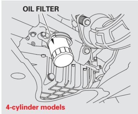
4. Install a new oil filter according to the instructions that come with it. Make sure to clean off any dirt and dust on the contacting surface of a new oil filter.
