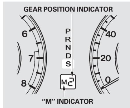
When you move the shift lever from "D" to "S" and pull either paddle shifter, the gear position indicator displays "M" along with the selected gear number.
