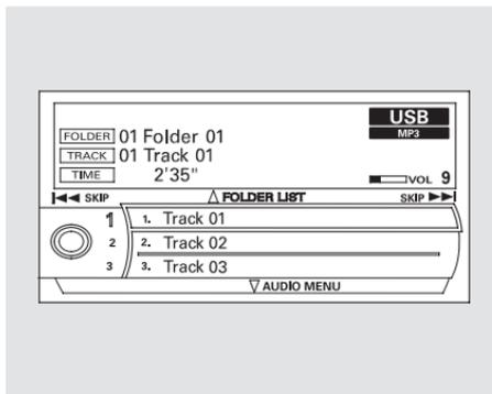
You can select any type of repeat, random and scan modes on the audio menu screen. Press the AUDIO button to show the audio control display on the navigation screen. Push down the selector on the interface dial to display the audio menu items.
