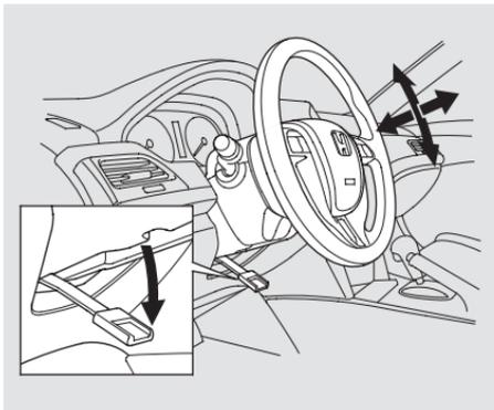
2. Move the steering wheel up or down, and in or out, so it points toward your chest, not toward your face. Make sure you can see the instrument panel gauges and indicators.
