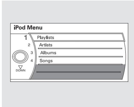
You can also select a file from any of the iPod menus: playlists, artists, albums and songs, by using the interface dial. Press the AUDIO button to display the audio control display on the navigation screen. Push up the interface selector to display the iPod menu. Turn the knob on the interface dial to select a desired list.
