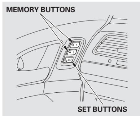
3. Press and release the SET button. You will hear a beep. Immediately press and hold one of the memory buttons (1 or 2) until you hear two beeps. The indicator in the memory button will come on. The current position of the driver's seat is now stored.
