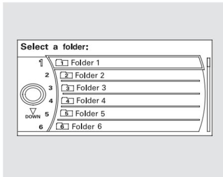
Push up the selector on the interface to switch the display to the folder list, then turn the knob on the interface dial to select a folder.
