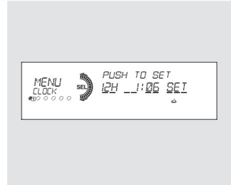
10. To enter the clock setting, turn the selector knob to select "SET," then press the knob. The display will return to the menu item display.
