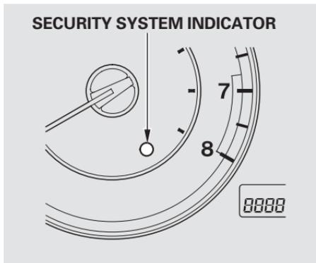
Once the security system sets, opening either door, the trunk, or hood without using the key or the remote transmitter, will cause the alarm to activate. It also activates if the ignition switch is turned to the ON (II) position, the audio unit is removed from the dashboard, or the wiring is cut.
