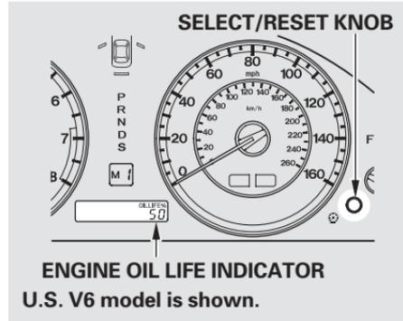
To see the current engine oil life, turn the ignition switch to the ON (II) position, then press and release the select/reset knob repeatedly until the engine oil life indicator appears (see page 64).
