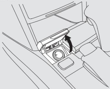
Your vehicle has two accessory power sockets; one is at the front of the center console and the other is in the console compartment.
