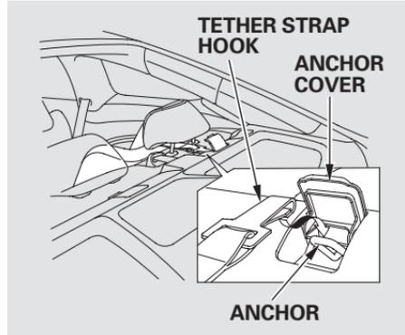
5. Lift the head restraint (see page 97 ), then route the tether strap through the legs of the head restraint and over the seat-back, making sure the strap is not twisted.
