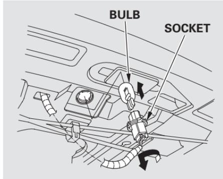
1. Open the trunk, and remove the socket from the light assembly by turning it one-quarter turn counter-clockwise.
