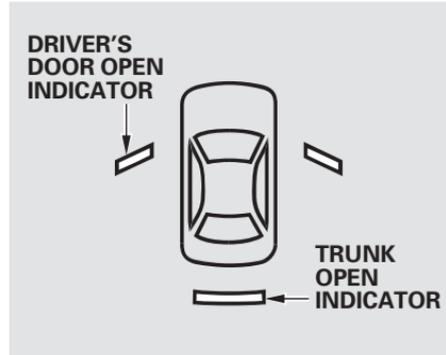
The appropriate indicator comes on if the trunk or either door is not closed tightly.
