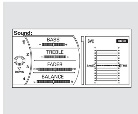
You can also adjust the sound by pushing the SOUND button repeatedly. Each mode is shown in the center display as it changes. Turn the power/volume knob to adjust the setting to your liking. When the level reaches the center, you will see "C" in the display.
