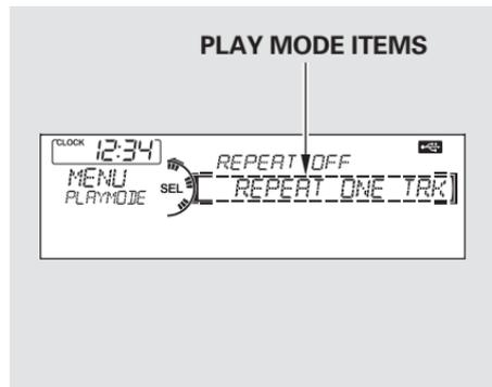
Turn the selector knob to select a play mode: normal play, shuffle off, shuffle all, shuffle album, repeat off, or repeat one track, then press ENTER to set your selection.
