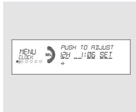
4. Turn the selector knob to select the item which you want to adjust. Turning the selector knob will change the selected item between the clock display setting, hours, minutes, and SET. The selected item is indicated with  $\Delta$  in the display.
