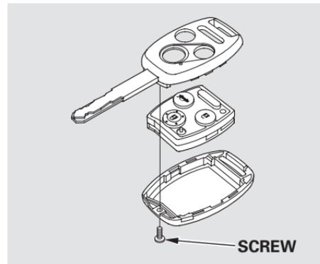
2. Separate the transmitter by prying its middle seam with your fingernail.
