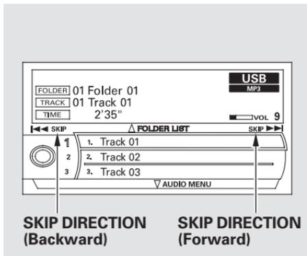
You can also change files with the interface dial. Press the AUDIO button to show the audio control display on the navigation screen. Push the selector knob to the right side to skip to the beginning of the next file, and to the left side to skip to the beginning of the current file. Pushing it to the left again skips to the beginning of the previous file.
