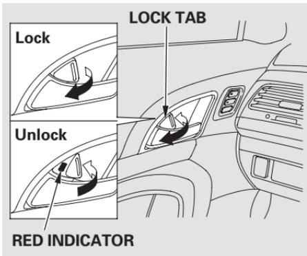
The lock tab on the passenger's door locks and unlocks that door.
