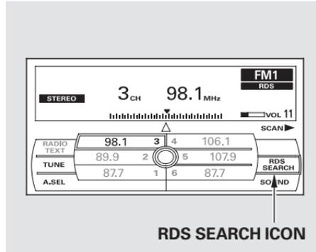
With the FM band selected, you can select the program type provided by the RDS. Press the AUDIO button to display the radio information on the screen. Push down the selector on the interface dial, then turn the knob to select RDS SEARCH icon. Press ENTER to set your selection. The principal RDS categories are shown as follows:
