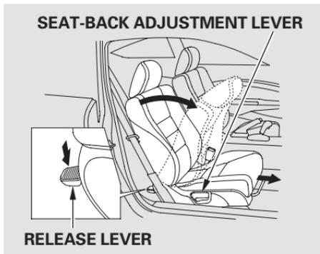
To get into the rear seat on the passenger's side, push downward on the release lever at the base of the seat-back, or pull up on the seat-back adjustment lever. The seat-back will tilt forward and the entire seat will move forward to allow easier entry to the rear seat.
