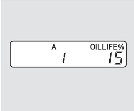
3. Press the select/reset knob for about 10 seconds. The engine oil life and the maintenance item code(s) will blink.
