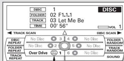
Using the interface selector, you can see the list of all the files and folders within a disc. While playing a MP3/WMA disc, press the AUDIO button. The currently playing folder and file information comes on the screen.
