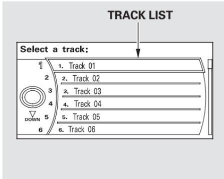
You can also choose a track directly from a track list. Press ENTER on the interface selector, and the track list screen will be shown. If there are no track names, track numbers are displayed. You will see the current track is highlighted. Turn the interface knob to select the desired track, then press ENTER on the interface selector.
