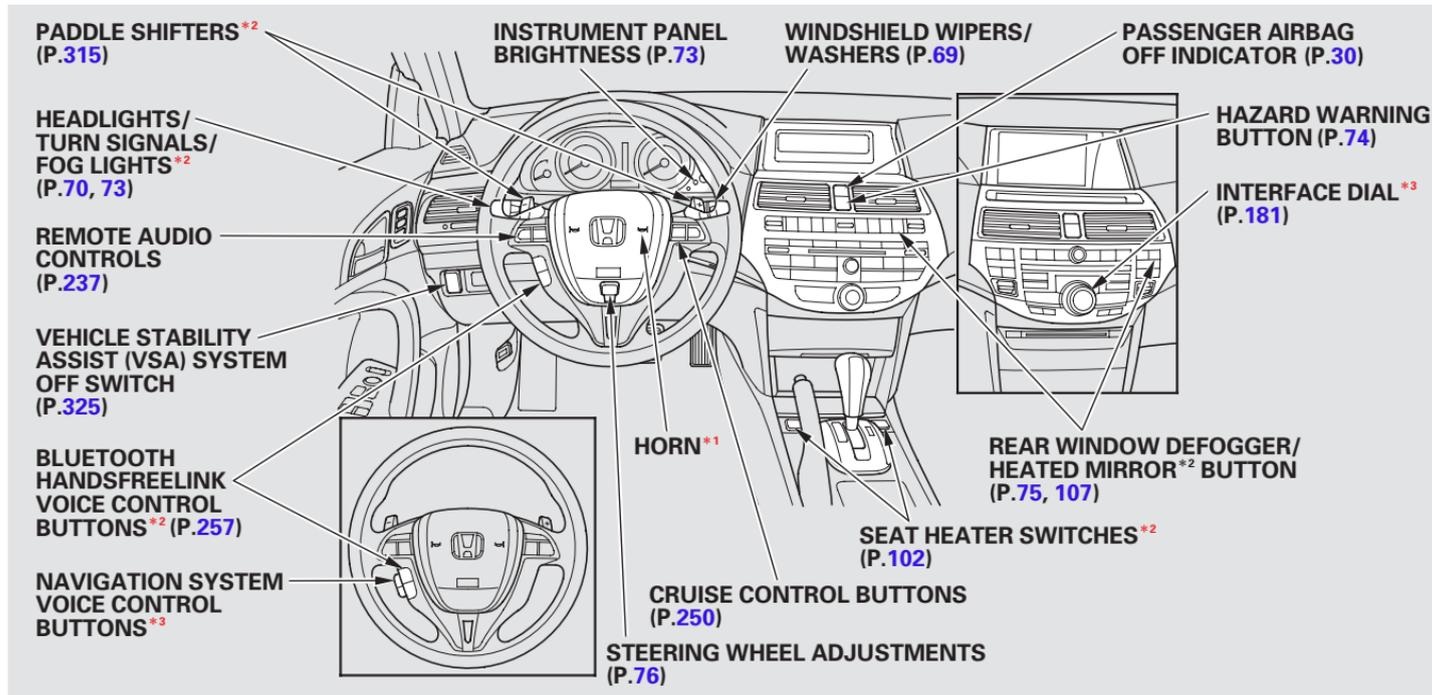
\*<sup>1</sup>: To use the horn, press the center pad of the steering wheel.
