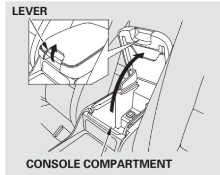
To open the console compartment, pull up on the lever and lift the armrest.
