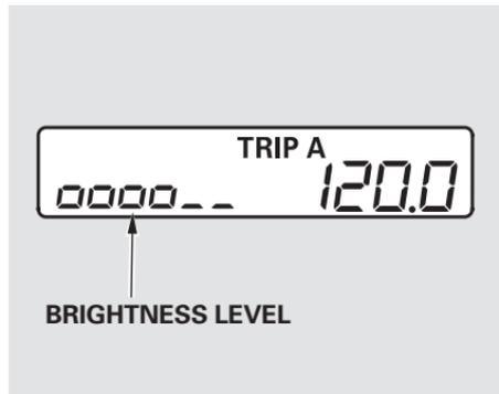
The level of brightness is shown on the information display while you adjust it. It goes out about 5 seconds after you finish adjusting.
