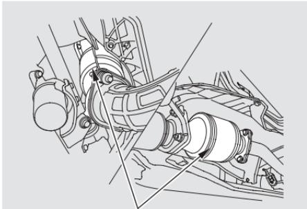
**THREE WAY CATALYTIC CONVERTERS**
