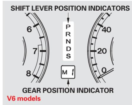
Using a paddle shift mode, the gear position indicator shows you the selected gear number (see page [315](#)).
