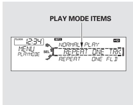
**REPEAT ONE TRK** – This feature continuously plays a file. Select normal play to turn it off. Pressing either side of the SKIP bar also turns off this feature.
