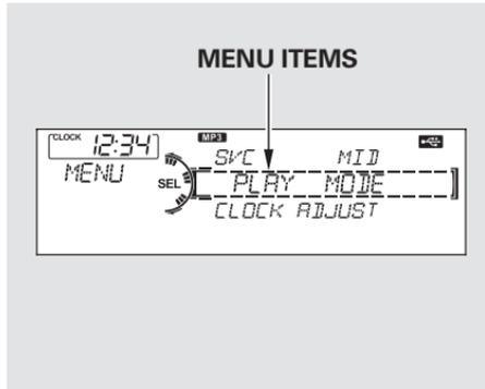
You can select any type of repeat, random and scan modes by using the MENU button and the selector knob. Push the MENU button to display the menu items, then turn the selector knob to select "PLAY MODE." Press the selector knob (ENTER) to set the selection.
