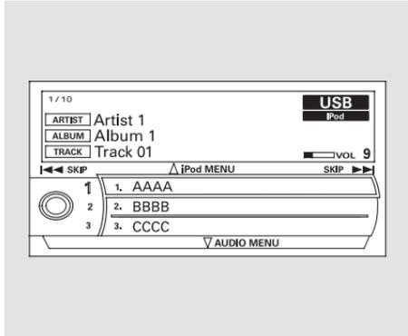
You can also change files with the interface dial. Press the AUDIO button to show the audio control display on the navigation screen. Push the selector to the right side to skip forward and to the left side to skip backward.
