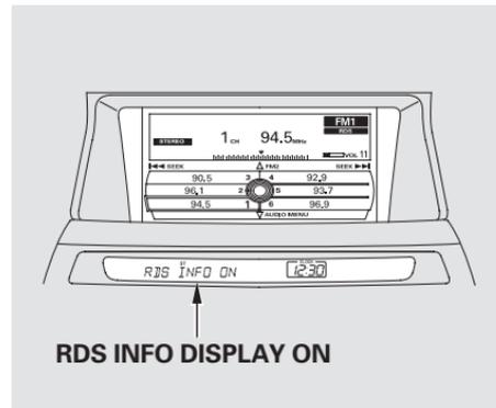
To switch the function between on and off, press and release the TITLE button. With the system on, you will see the “RDS INFO ON” message on the display. If the station you are listening to is an RDS station, the display shows the station name.
