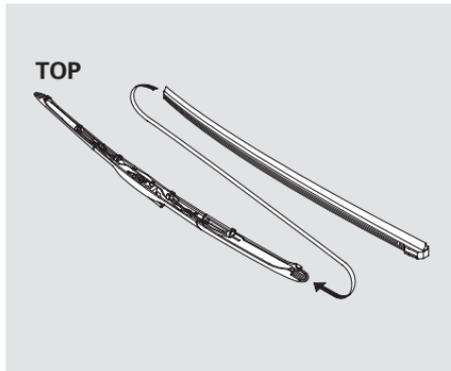
5. Place the top of the wiper blade on the end of the blade assembly, and slide the blade onto the assembly until the tabs are fitted onto the wiper blade.
