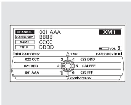
To listen to XM Radio, turn the ignition switch to the ACCESSORY (I) or ON (II) position, and press the (« XM ») button. The last channel you listened to will show in the audio screen and the center display. Adjust the volume by turning the power/volume knob.
