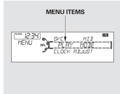
You can select any type of repeat and shuffle mode by using the MENU button and the selector knob. Press the MENU button to display the menu items, then turn the selector knob to select "PLAY MODE." Press ENTER to set the selection.
