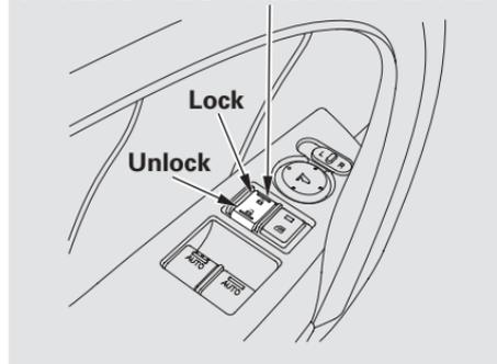
To lock both doors, push the front of the master door lock switch on either door, pull the lock tab rearward on the driver's door, or use the key on the outside lock on the driver's door.
