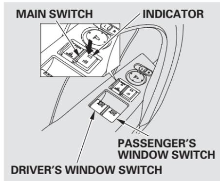
Turn the ignition switch to the ON (II) position to raise or lower either window. To open a window, push the switch down and hold it. Release the switch when you want the window to stop. Pull back on the switch and hold it to close the window.
