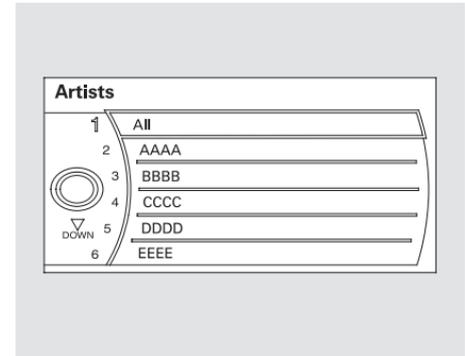
Push ENTER on the selector to display the items on that list, then turn the knob on the interface dial to select a desired list. Pushing the selector up or down moves a selection to the top or bottom of the screen items. Press ENTER to set your selection.
