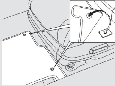
The driver's and right rear passenger's floor mats that came with your vehicle hook over the floor mat anchors. This keeps the floor mats from sliding forward and possibly interfering with the pedals (driver's floor mat) or with the seat weight sensors (right rear floor mat).
