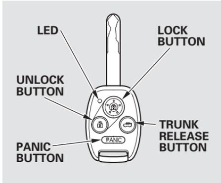
**LOCK** — Press this button once to lock both doors. Some exterior lights will flash once. When you push LOCK twice within 5 seconds, you will hear a beep to verify that the doors are locked and that the security system has set. You cannot lock the doors if either door is not fully closed or the key is in the ignition switch.
